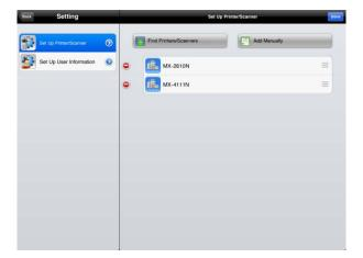
VIII. Tapping enables user to delete a printer/scanner from the list.
