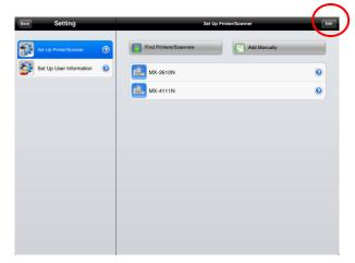
VII. Tapping "Edit" button enables user to delete and arrange order of the printer/scanner.
