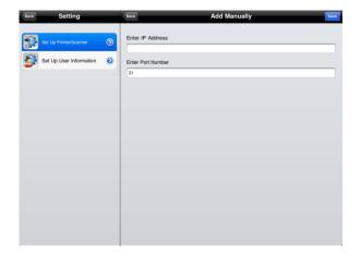
X. Enter IP address and port number to add a printer/scanner.
