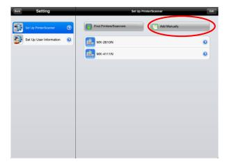
IX. Tap "Add Manually" if you wish to add any printers/scanners that cannot be added on "Find Printers/Scanners."
