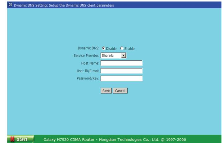
Before enabling the dynamic DNS function, you should apply a valid account from a service provider in the drop list. Input the following information.
