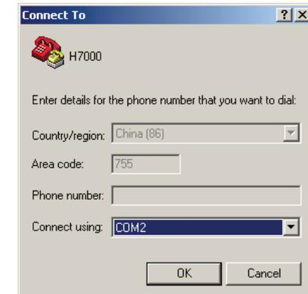
The COM port parameters should be specified. Select COM number (i.e. COM2), Bites per second, Data bits, Parity, Stop bits and Flow control.
