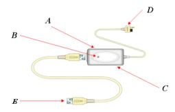
A. This is equipment that converts data to download from user's PC to audio card. The file can be saved in the speed of maximum 0.8 Mbps.
