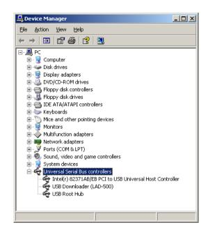
If USB driver is installed successfully, "USB Downloader(LAD-500)" is shown in [Device Manager] as the picture above.
