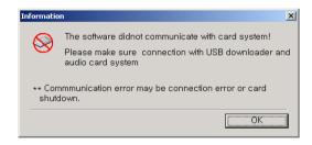
This is the error message taken place when do the function related to audio card while the card is not connected. In this case, check the connection with audio card and the USB downloader.
