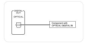
You can enhance the sound quality be connecting this OPTICAL DIGITAL OUT to the OPTICAL DIGITAL IN of an amplifier, MD recorder, etc.
