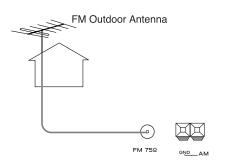
• A  $75\Omega$  outdoor FM antenna may be used to further improve the reception. Disconnect the indoor antenna before replacing it with the outdoor one.
