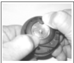
Fig. 82 - Retaining Ring Tabs
