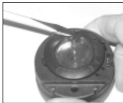
Fig. 77 - Hatch Ring Removal
