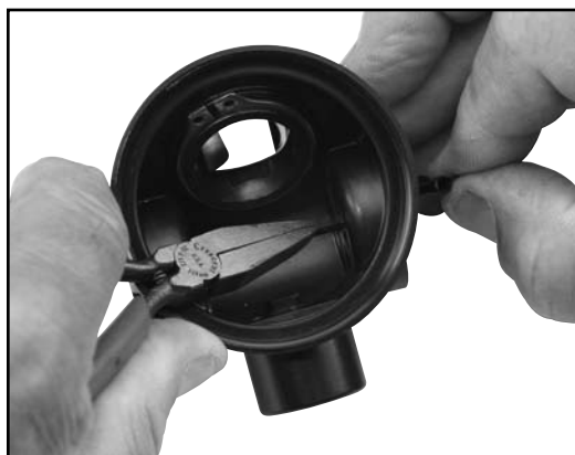
3) Removal of Exhaust Valve
