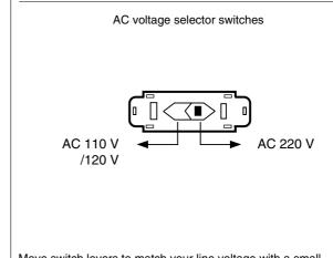
Move switch levers to match your line voltage with a small screwdriver or other pointed tool.
