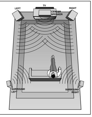
*Note :* to avoid interference with the TV picture, use only magnetically shielded front speaker systems.
