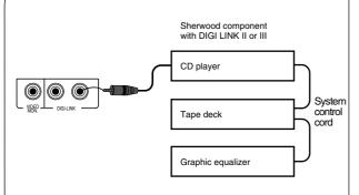
Connect this jack to the DIGI LINK jack of the external Sherwood component that uses the DIGI LINK II or III remote control system.
