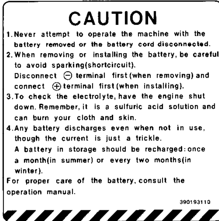
CAUTION - Battery PART NO. - SBA-390193110 LOCATION - Inside of front hood
