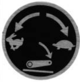
Row Control valve PART NO. - SBA-390370290 LOCATION - Top of flow control knob
