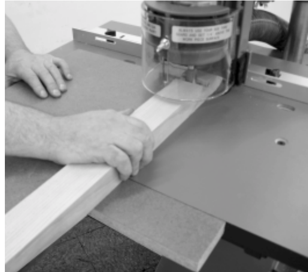
Figure 32. Cutting a dado across the grain with a wooden pusher. Guide stock against the Fence.
