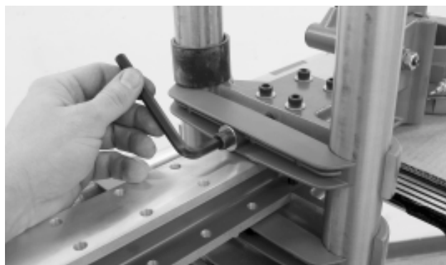
Figure 3. Tighten the Clamp cap screws with the 5/16" Allen wrench.
