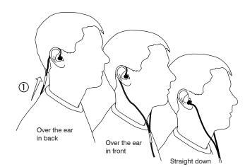
Tighten the cable and take up slack by raising the cable sleeve ①.
