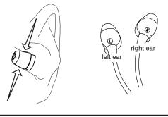
Make sure that the sleeve completely covers the earphone nozzle. If any part of the nozzle is exposed, the sleeve is not properly installed.
