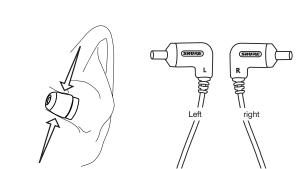
Warning: Do not push the earphone sleeve beyond the ear canal opening. Make sure that the sleeve completely covers the earphone nozzle. If any part of the nozzle is exposed, the sleeve is not properly installed.
