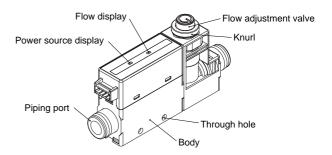
Power source display (green): Turns on when power is supplied.
