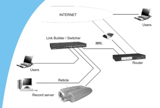
For this program, not only the basic setup of PC and IP camera but also the setup of Port Forwarding function of Router is required, so the visit for network camera besides Intranet is accessible. The Router should have the function of Network Address Transition(NAT) to transit the global address to local address and assign the different external port No. to each IP camera.
