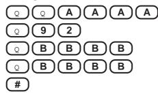
Where AAAA represents the old 4-digit PIN code and BBBB represents the newly chosen 4-digit PIN code. To confirm correct input of your PIN code the siren will bleep after entering the last digit. The number 92 is the access code/command which notifies the alarm unit to accept the new PIN code.
