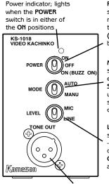
POWER switch: three settings: ON is on, with no buzzer, OFF turns the unit off, and ON (BUZZ ON) uses the built-in buzzer
