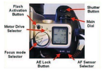
Figure 3: Focus Mode Switch
