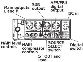
**MAIN outputs L and R** Balanced XLR-3 connectors providing the main analog output signals from the KS-342. They can also be used to provide the outputs from input channels 1 and 2, for example when these are used in MS mode.
