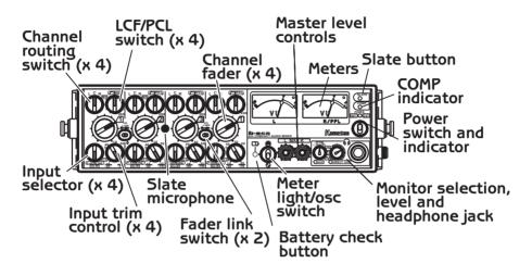
**Channel routing switch (x 4)** Each channel has a switch that allows the channel's output to be routed to either the left (L), right (R) or both (C) output busses.
