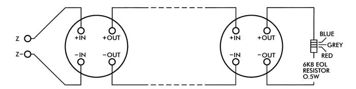
Line continuity unit wiring. Diode bases are used. Removal of a detector indicates fault and detectors beyond the removed one remain operative.
