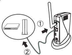
Connect a network cable to this product. Connect the other end of the network cable to a network hub, switch, or router.
