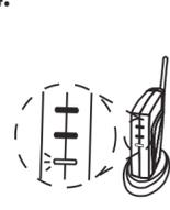
Verify the Link LED (Green) turns on and the Wireless LED (Green) turns off.
