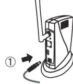
Connect the AC adapter to this product and the power plug to the outlet.
