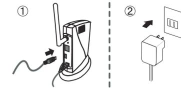
Connect the printer to be shared over the network along with this product via a USB cable and insert the power plug of this product into the outlet.
