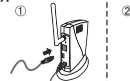
Connect the printer to be shared over the network along with this product via a USB cable and insert the power plug of this product into the outlet.
