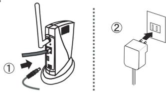
Connect the AC adapter to this product and the power plug to the outlet. (Do not connect the printer to this product yet. Printer will need to be connected at '17'.)
