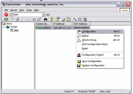
6. The IP Address settings of the SX-600 are for configuration purposes only. These will not effect the network device you are connecting to. You do not normally need to change these settings if you want to continue to make future configuration changes by connecting directly from a PC with a crossover Ethernet cable.
