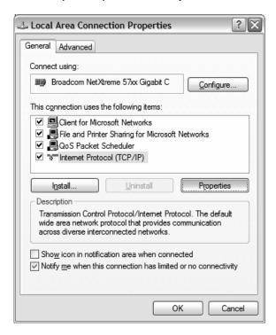
4. Select *Obtain an IP Address Automatically* in the TCP/IP properties and click *OK*, then *OK* again.
