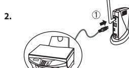
Connect the USB devices to be shared over the network along with this product via a USB cable2.
