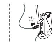
To reflect the wireless configuration, disconnect the power plug from the outlet and unplug the network cable. Do not unplug the network cable when using this product with a wired LAN.
