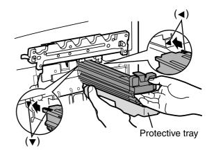
$\boldsymbol{8}$  Install the waste toner cartridge (1) and slide the lock lever to the left (2).
