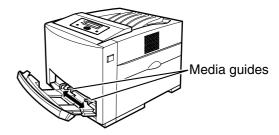
*3* Insert media with the **printing side down** into the multi-purpose tray while adjusting the media guides to the media width.
