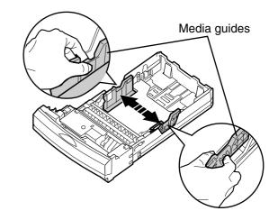
3 Slide the length guide unit to adjust it to the media length. Slide the length guide unit (2) while pressing the PUSH mark (1) to extend it.
