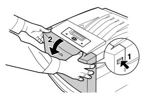
2 Insert the automatic duplex unit while confirming the position (A and B).
