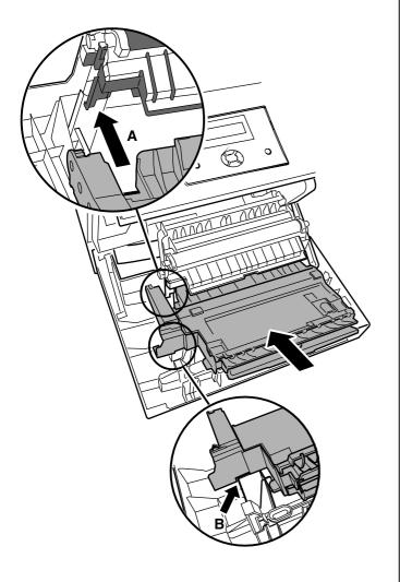
*3* Push the automatic duplex unit down (1) (and paste the label (2) provided with KX-CL400 only so it is overlapped on the jam clear label that has been pasted).
