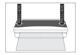
Press and hold the Seal/Cut button 3 with both hands until the control lamp 3 lights up. Hold the Seal/Cut button 5 pressed down until the control lamp down 3 goes out.
