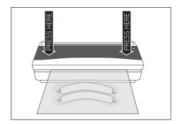
As soon as the air has been sucked from the bag, press and hold the Seal/Cut button with both hands, as already described, and seal the bag.
