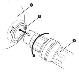
◆ Afterwards, insert the hose fitting on the other side of the air hose <sup>❸</sup> firmly into the connection-support of the air-bubble mat **2**.
