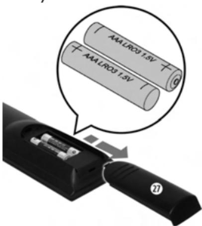
1. Open battery compartment cover ②⑦ in the direction of the arrows.
