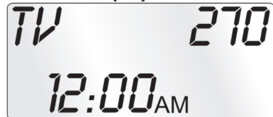
The standard display of the LCD display ❶ consists of details of the current device, i.e. "TV", the device code and the time of day.
