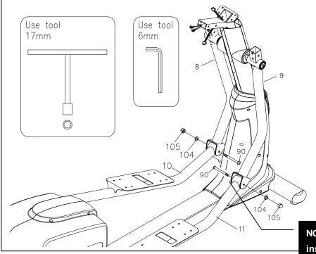
Note: make sure the bolts are fully tightened to avoid noise
