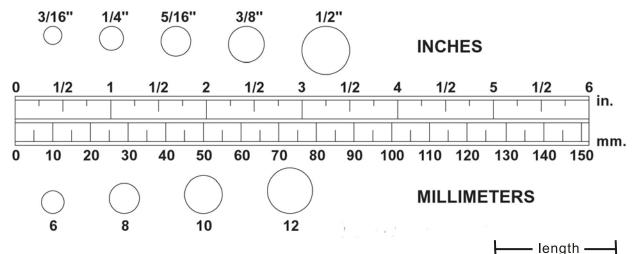
**NOTE:** The length of all bolts and screws except those with flat heads is measured from below the head to the end of the bolt or screw. Flat head bolts and screws are measured from the top of the head to the end of the bolt or screw.
