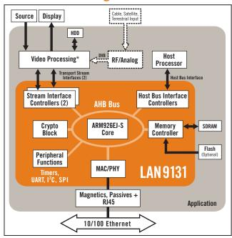
\* Depending on the application, video processing can include a video decoder or encoder, MPEG PID filter or other conversion functions
