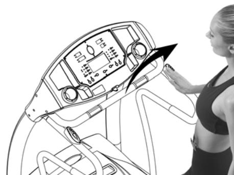
3. Wave you left hand approximately 6 inches above the motion sensor on the left handle bar to decrease the speed. The sensor will sound one short BEEP per scan and decrease speed by 0.1 MPH. Holding your left hand approximately 6 inches above the left sensor constantly results in the sensor sounding one long BEEP per second and decreasing speed by 0.5 MPH per second.
