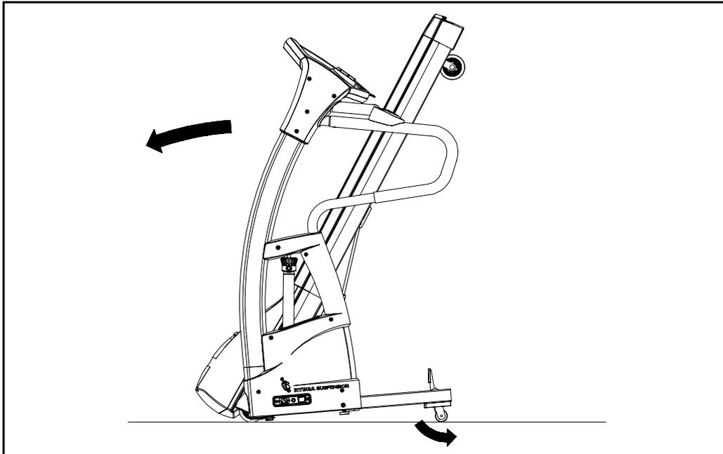
**Lift the deck from the rear so that the treadmill rests on the front transportation wheels.**
