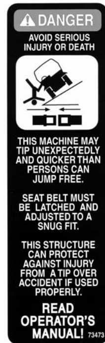
DANGER – OPERATOR PROTECTIVE STRUCTURE
