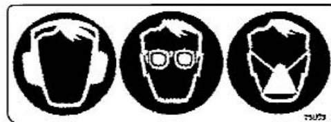
75893 - EAR/NOSE/BREATHING PROTECTION REQUIRED - LOCATED ON SIDE OF BLOWER HOUSING
