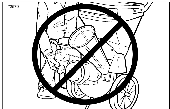
Figure 15. Improper Lifting Of Unit
