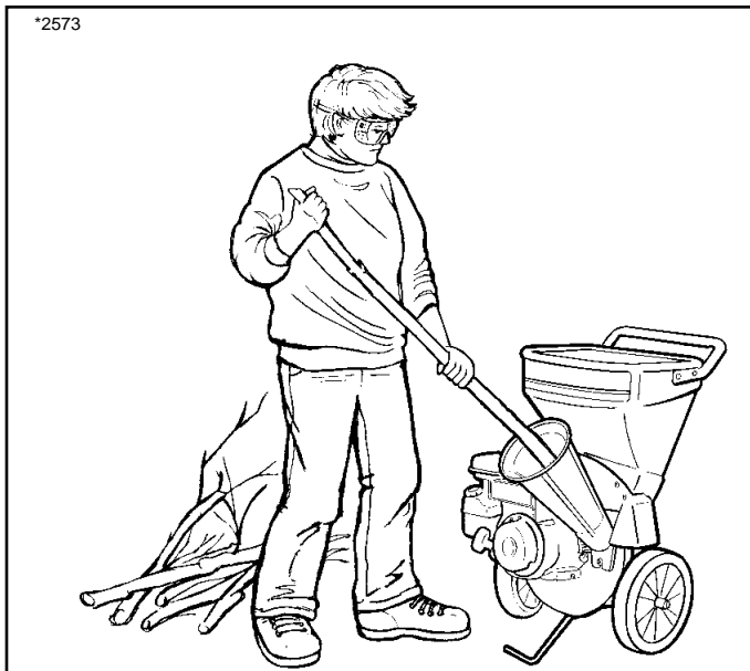
Figure 7. Proper Stance for Chipping
