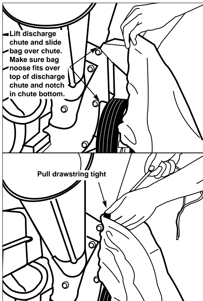
Figure 5A. Discharge Bag Installation
