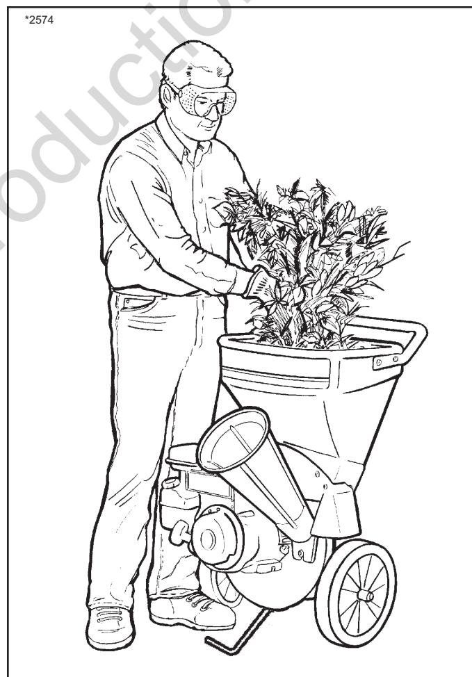
Figure 9. Properly Feeding Longer Materials for Shredding
