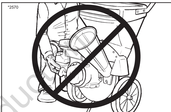
Figure 15. Improper Lifting Of Unit
