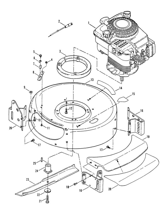
Engine, Cutting Deck, Blade, Interlock (Push Models)
