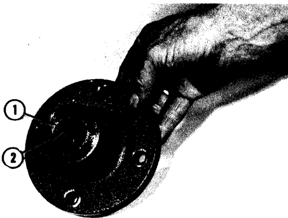
FIG. 10.7--BEARING AND SEAL INSTALLED
