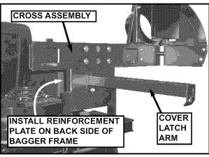
**STEP 14:** Install cross assembly onto bagger frame with four 3/8-16 x 3/4 bolts and hex flange lock nuts, tightening securely. Insert bolts back through bagger frame and into cross assembly.
