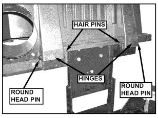
**STEP 16:** Lay cover assembly on cross assembly. Align hinges on cross assembly with hinges on cover, and install one round head pin through each set of hinge holes, securing with a hair pin.
