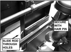
**STEP 14:** Slide hitch rod through aligned holes in clamshell mount and bumper mount plate, securing with hair pin.
