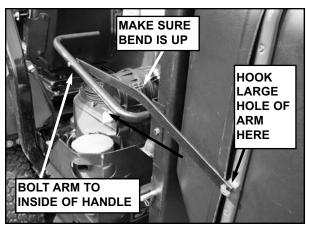
**STEP 15:** Hook the large hole of each actuating arm onto the hook on each side of the rear cover. Then secure the other end of the arm onto the inside of each side of the handle weldment with one 3/8-16 x 2" hex bolt and nyloc nut. Tighten snugly. **NOTE:** Make sure bend of arm is up.
