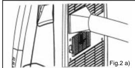
c.) Connect the window kit adaptor to the external end of the exhaust duct for a window or sliding door hot air outlet installation.
