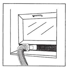
c) Or connect the window kit adaptor to the external end of the exhaust duct for a window or sliding door hot air outlet installation.
