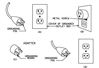
**WARNING**: This heater is for use on 120 volts. The cord has a plug as shown in A. An adapter as shown in C is available for connecting three-blade grounding-type plugs to two-slot receptacles. The grounding lug extending from the adapter must be connected to a permanent ground such as a properly grounded outlet box. The adapter should not be used if a three-slot grounded receptacle is available.
