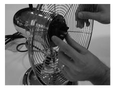
Position the back grille over the motor shaft, aligning the holes in the back grille with the two knobs that protrude from the motor. Make sure the handle is at the top.
