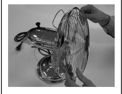
Position front grille so logo is horizontal. Secure the top tab to the back grille. Snap the two remaining metal clips to complete the assembly.
