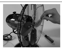
5) Slide the fan blade onto the mounting shaft with the shaft sleeve facing the motor. Align securing screw with flat groove in the motor shaft and tighten with Phillips screwdriver.
