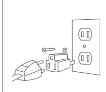
WARNING: This heater has a grounded three pronged plug intended to fit into a three slot outlet. An adapter is available for connecting three pronged plugs into two slot outlets. When doing so, the green grounding tab extending from the adapter must be fastened under the wall plate's mounting screw. The adapter should not be used if a three-slot outlet is available.
