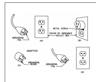
WARNING: This heater is for use on 120 volts. The cord has a plug as shown in A. An adapter as shown in C is available for connecting three-blade grounding-type plugs to two-slot receptacles. The grounding lug extending from the adapter must be connected to a permanent ground such as a properly grounded outlet box. The adapter should not be used if a three-slot grounded receptacle is available.
