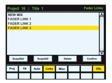
To set up a new link, scroll to **New Link** and press the D-pot push switch. This will create a new entry in the list suffixed with a number. This entry will be automatically highlighted, and faders can be added to (or removed from) the link by pressing their **fader** buttons. Link numbers are shown in the fader scribble strip and the red fader status LEDS will indicate those faders in the currently selected link.
