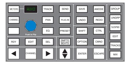
The majority of functions are controlled via dedicated buttons with less reliance than the HUI interface on the 8x8 menu button matrix located beneath the TFT screen. When compared to the HUI front panel, the main changes are as follows:
