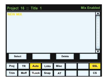
Now press the encoder switch to select the New Mix Setup page (see below). All the channel faders will enter Absolute mode, as indicated by a red LED next to each fader.
