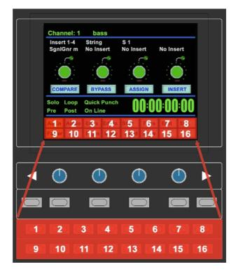
The top row (buttons 1-8) allows selection of the labelled functions. Once pressed, a submenu will appear below. These items are selected using the second row of soft key buttons (9-16). The menus are ordered as follows:
