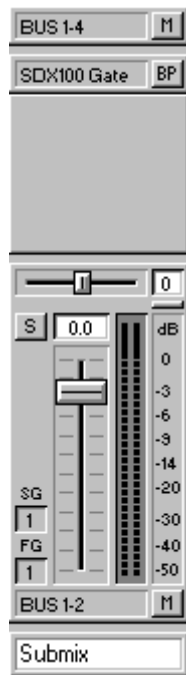
A typical 4 in - stereo out mixer column, as seen within the Mixer.
