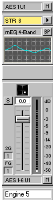
A mono in - mono to 5.1 out mixer column, as seen within the Mixer.
