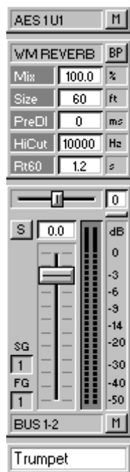
A typical mono in - stereo out mixer column, as seen within the Mixer.
