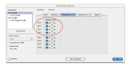
In the Hardware Setup window, the "Output Trim" settings are irrelevant to the Delta-Link MADI HD because its inputs and outputs are all digital. Therefore, they can be used to set various Alpha-Link parameters as follows:
