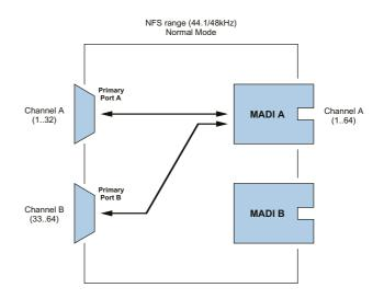
NOTE: The MADI Port B output signals duplicate the MADI Port A output signals, but the MADI Port B inputs are not connected internally to the Primary Ports in this mode.
