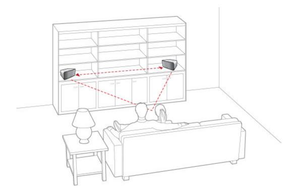
**Note:** The Stereo Pair setting is for use with PLAY:3 and PLAY:5 units only. Both Sonos components in the stereo pair must be the same.
