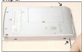
Remove the two Phillips screws from the upper sides of the device, as shown, using the same mini flathead screwdriver or a 000 Phillips screwdriver. Set the screws aside for reassembly.
