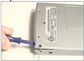
Use the plastic flathead screwdriver or any small flathead screwdriver (plastic recommended - metal may scratch) to separate the back case from the front by CAREFULLY prying around the device. There are clips on all sides of the device holding the front and back together. Be careful not to break them when prying.
