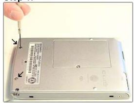
Remove the two "Y Head" three pointed screws below the label on the back of the device, as shown, using the included mini flathead screwdriver. (Your tools may look different than the picture shown.) You can also use a "Y Head" screwdriver if you have one. Set the screws aside for reassembly.
